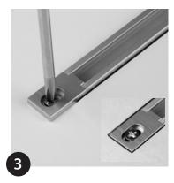
Can be installed semi-recessed as shown, fully recessed flush OR into specific s/steel handrail hardware - Consult with your handrail manufacturer/supplier before specification. For flush install L12mm Nylon spacer washers would be recommended under each end cap.
